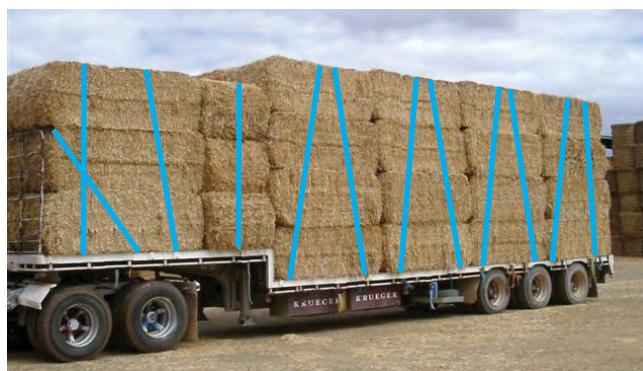
Figure 9.4 The use of a diagonal bracing strap improves load stability. Diagonal bracing should be considered for at least the front and rear groups of bales on a trailer, with the bracing pulling towards the centre of the trailer. Diagonally bracing all groups of bales with two straps is also acceptable – source ARRB Group, 2006.
